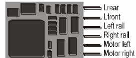
MX620 Micro processor side shown (connector pins are soldered to other side !)
